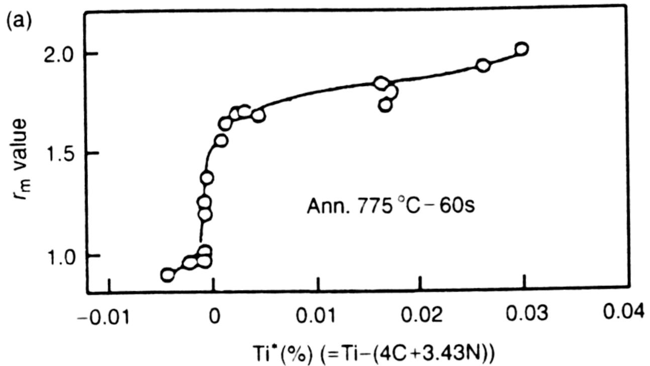
**But excessive Ti causes surface defects!**
